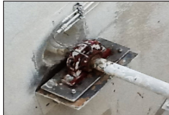
Chesterton 630 SXCF grease is now injected remotely to 3 lube points per bearing.
